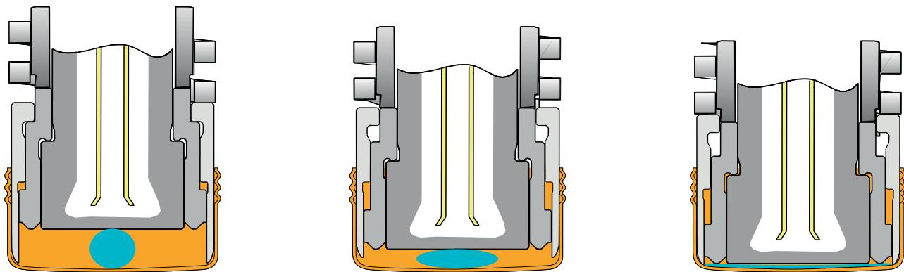
**EN** By using non-PVC raw materials the lining machine is able to form the liners directly inside the cap shell.
